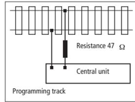
When programming using Lenz, Uhlenbrock or Arnold equipment, please refer to their programming instructions. If the error message "err02" is displayed during programming with Lenz or Arnold equipment, a 47 Ohm resistor (0.5 Watt or higher) must be inserted between one of the two supply cables and the programming track.
